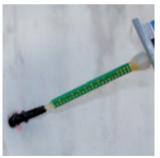
Insert static mixer into the packer nozzle with light pressure. Inject.
