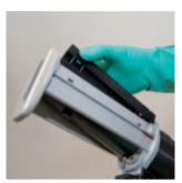
1. Loosen and remove the cartridge sleeve by pressing the clips together.
