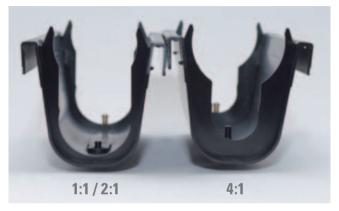
The MC-Fastpack Power-Tool is pre-set with the cartridge sleeve for cartridges with mixing ratio 1:1 and 2:1.
