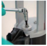
2. Loosen both screws and remove plungers.
