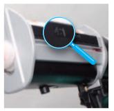
Check cartridge sleeve for the correct mixing ratio.
