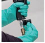
2. Adjust injection pressure at the pressure limiting valve.
