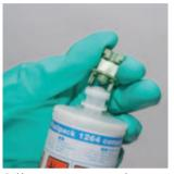
Unscrew cap nut and remove the plug from the cartridge.
