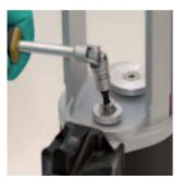
According to the required cartridge sleeve, use the matching plungers and tighten the screws.
