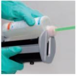
4. Insert cartridge into the MC-Fastpack Power-Tool.
